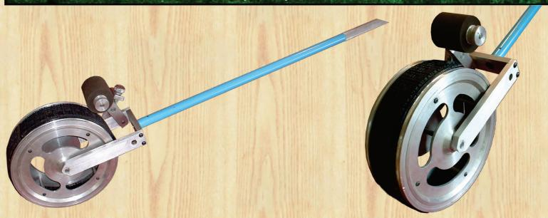
The **G-22 Printer** is designed for off-line application of panel stamps and is made with a lightweight, aluminum alloy handle. Rolls easily across any panel surface leaving clear, crisp impressions. The print drum has a print area equal to most industrial line printers and Velcro mount for easy stamp changes. Comes with print wheels of various diameters and widths to fit any size stamp.
