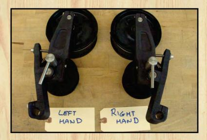
The **G-Series** are medium duty line printers designed to provide continuous impressions from a friction driven stamp wheel. The stamp hub has a rubber bumper on one side to absorb any shock and allow smooth application of stamp impression. These printers can be mounted directly above, beside, (left or right) or below the production line. The ink roll assembly snaps on and off with ease for quick, no mess changing of ink rolls.
